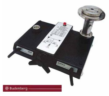
Pneumatic Dead-Weight Testers. Primary standards for Pressure Calibration
